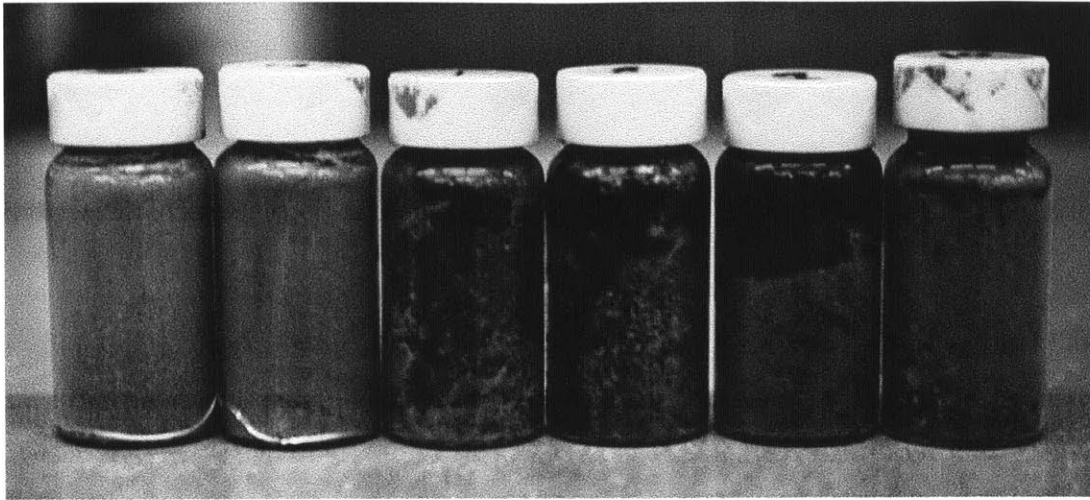
Figure 3-14: Comparison, from left to right, of pairs of vials of the optimal mixture (with cracks), Portland cement, and a sub-optimal mixture containing magnesium oxide that was not able to crack its container. Dye penetrant placed into the uncracked vials reveals that dye flows in channels along the outer surface of the Portland sample while it undergoes a diffused or retarded flow in the sub-optimal mixture. This indicates that MgO is adequate at providing even a baseline resistance to gap flow.
