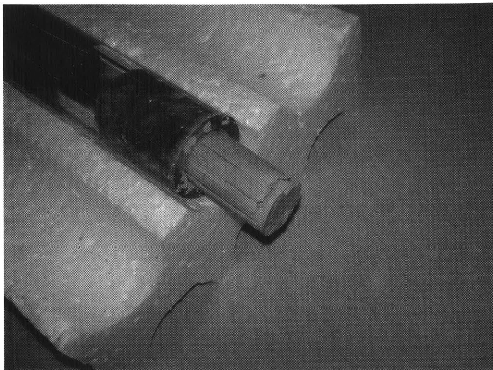
Figure 5-7: Sample #5 of freshly prepared 70/30 Bentonite/Water protruding after being heated in a furnace at 150 °C for 15 minutes.
