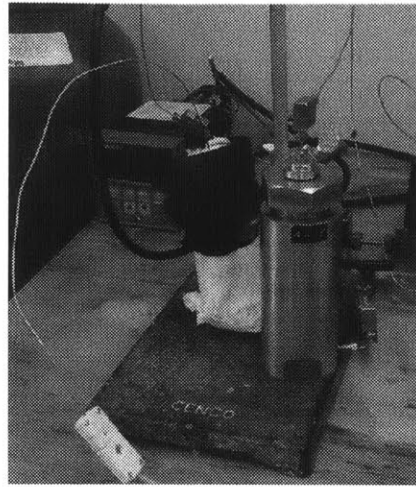
(b) The pressurized sample was prepared in a small quantity. It was held at 200 bar within this steel piston for 6 days, after which CO_2 bubbles were observed dissolved in the surrounding water.
