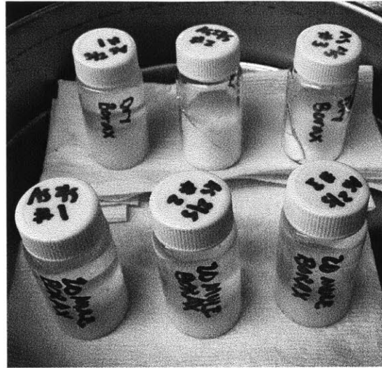
Figure 3-4: Top Row: Three vials of anhydrous sodium tetraborate left in contact with a head of water overnight. All three would eventually crack. Bottom Row: Hydrated borax left overnight with the same conditions. All three samples retained a “slushy” consistency.
