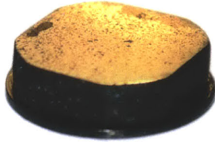
Fig. 3.3. Typical polished clinker sample. After epoxy impregnation and cutting, samples are glued on AFM disks, automatically leveled and manually polished to a mirror-like surface.
