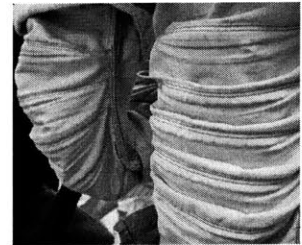
A detail of the current EMU's restraint layer around the knee joint.
