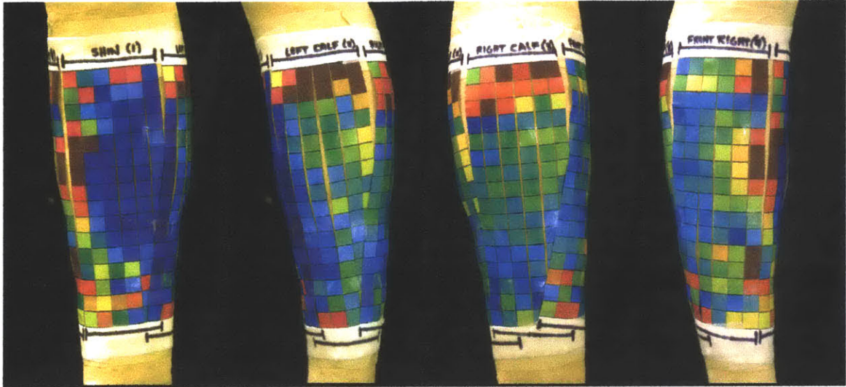
Figure 9.30: Photos of the average pressure data applied to the 3D print. Each point represents the data averaged across repetitions and days.
