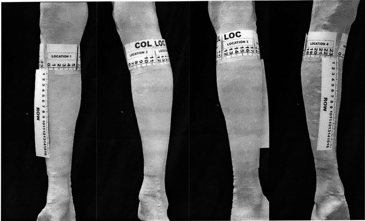
Figure 9.24: Photos displaying the sensor locations, one through four, the column-locations, zero through twenty three, and the rows, one through sixteen. The combination of the row number and the column-location number uniquely determine the location of each sensing element.
