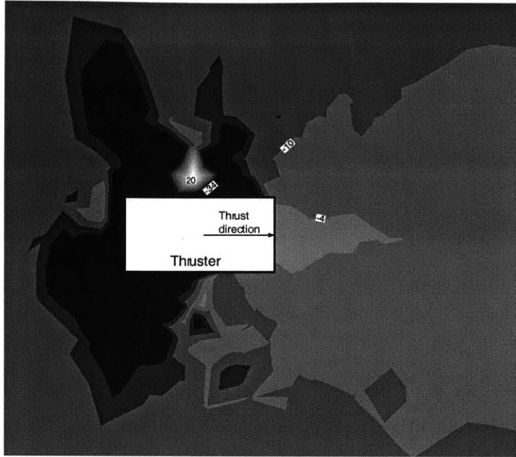
Figure 4-6: Potential contour at a snapshot in time showing a numerical instability.
