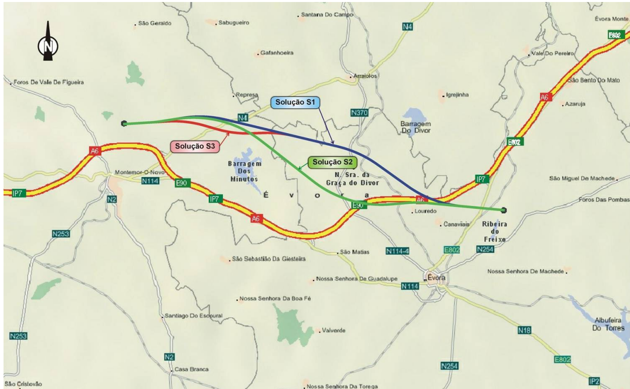
Figure 4-2 Évora HSR Environmental Impact Study – a single station option and multiple alignments (Source: RAVE 26 )
