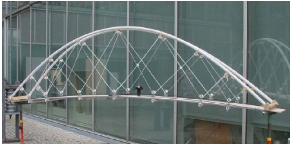
Figure A.10: Model of a tied-arch bridge with a pre-stressed arch in GFRP (photo: Jülich [27])
