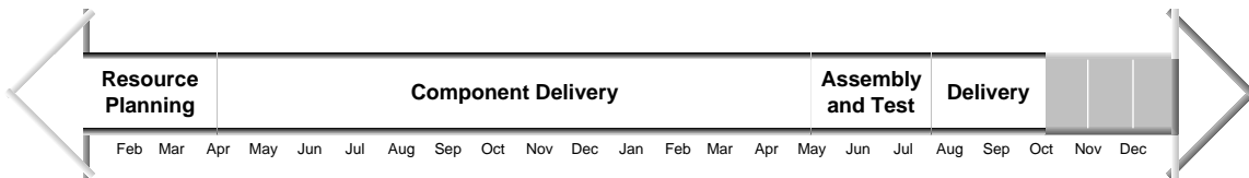
Figure 2-3 Typical Missile Manufacturing Timeline
