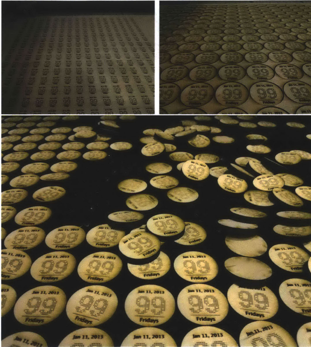
Figure 5-4: The fabricated tokens on the laser cutter bed after being manufactured. Each token has 32 bits of unique identifying information.
