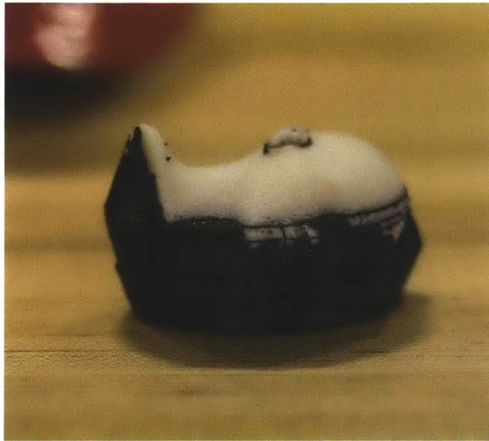
Figure 6-11: 3D printed result of using a bad mesh model.
