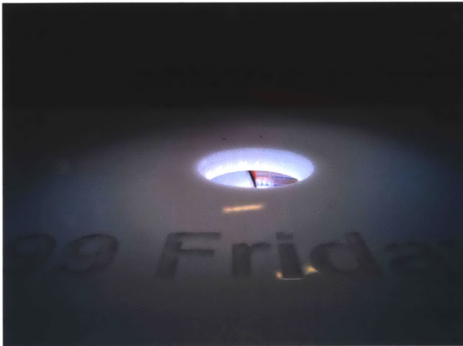
Figure 5-5: A close up showing the illuminated opening of the final token reader.
