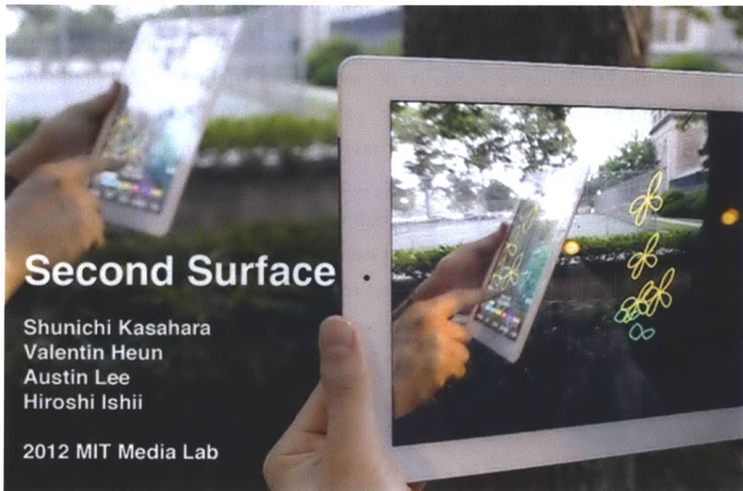
Figure 20: Second Surface system allows users to collaboratively place drawings, texts, and photos three-dimensionally in physical locations using tablet-based AR technology.
