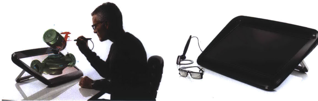
Figure 17. zSpace combines a stereoscopic 3D screen with a tracked pen-like device. This allows a user to manipulate virtual 3D objects precisely. Image courtesy of zSpace.
