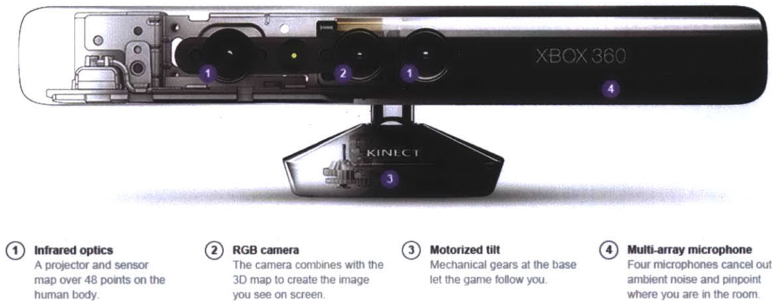
Figure 31. The Microsoft Kinect sensor captures a color as well as a depth image in the resolution of 640x480. Image courtesy of Microsoft.
