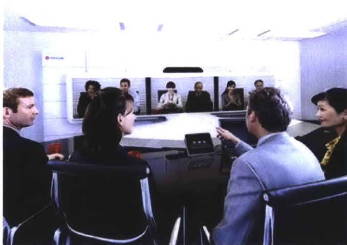
Figure 4. This image shows Polycom's telepresence system. It allows remote collaborators to sit together at a round table. Image courtesy of Polycom.
