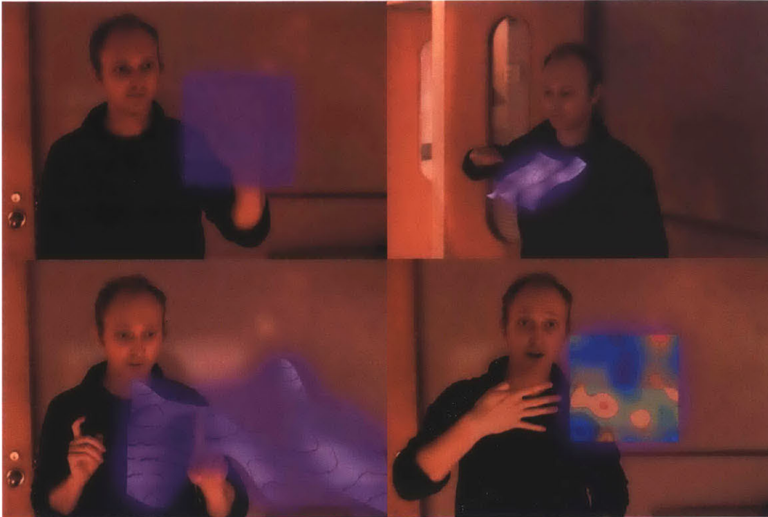
Figure 15. ARCADE (Stein, Xiao, Tompson, Hendee, Perlin, & Ishii, 2012) is a system that allows real-time video-based presentations that convey the illusion that presenters are directly manipulating holographic 3D objects with their hands. Image courtesy of Stein, Xiao, Tompson, Hendee, Perlin and Ishii.
