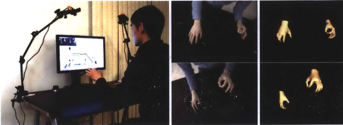
Figure 19. 6D hands is a bimanual hand tracking system that provides physically-motivated 6-DOF control for 3D assembly. Image courtesy of Wang, Paris and Popovic.
