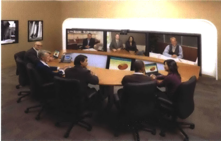
Figure 3. Cisco's telepresence room extends a round table into the remote spaces to have participants sit at the same table. It uses high-definition video and audio. Image courtesy of Cisco.
