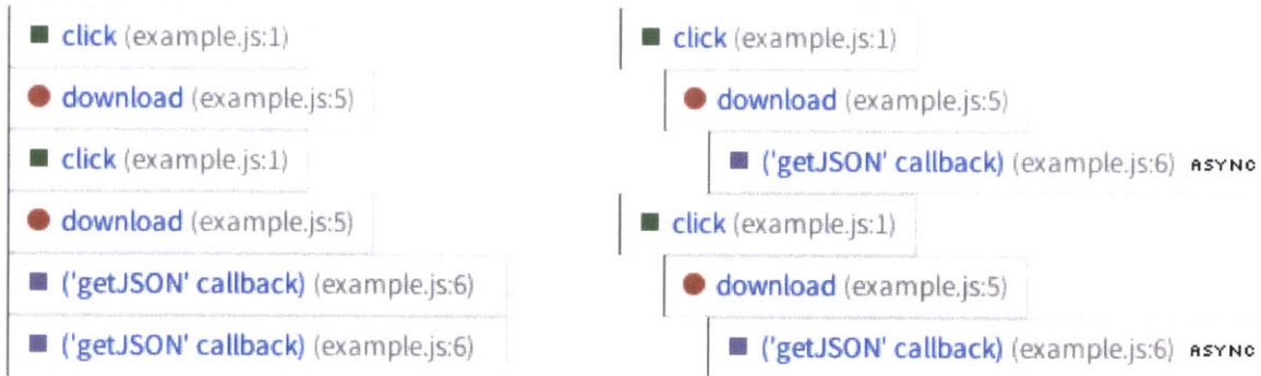
Figure 3-3: How the structured log is constructed. Left: a flat, chronological log, as you would get by adding print statements. Right: a structured log shows the call tree. In this example, download() calls getJSON (not in the log), passing a callback handler for when the download finishes. The responses come back out of order and would require the programmer to deduce which response goes with which request, but the structured log treats the asynchronous operation as a synchronous call for visualization.
