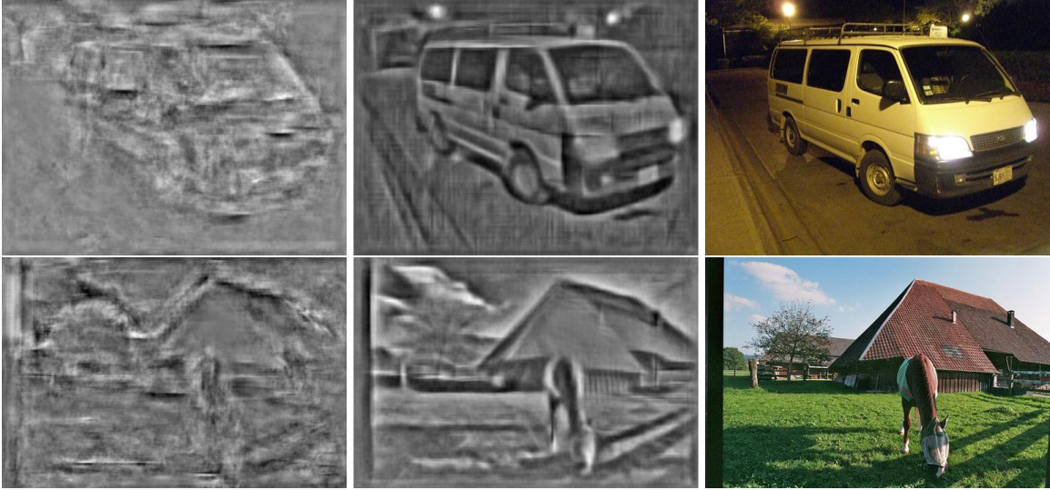
Figure 5-6: We invert only the texture features inside HOG and compare to the full HOG reconstruction. Left: texture only visualization. Middle: full HOG visualization. Right: original image. Even though the texture features are very low dimensional (4 dimensions per cell), there is still significant information stored inside.
