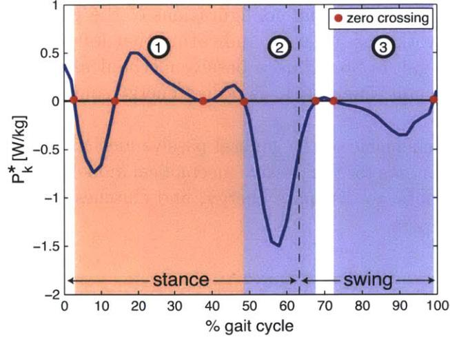
Figure 4-3: The three phases of gait. Power versus time graph is shown for a prosthetic leg with a typical inertial configuration (upper leg mass = 50% of able-bodied value, and lower leg and foot mass = 33% of able-bodied values) moving with normative kinematics at a natural cadence.  $P_k^*$  is power normalized by body mass. Phase 1 is an energy dissipation and generation phase ( $\frac{E_{diss}}{E_{gen}} = 0.77$ ), and phases 2 and 3 are energy dissipation phases.
