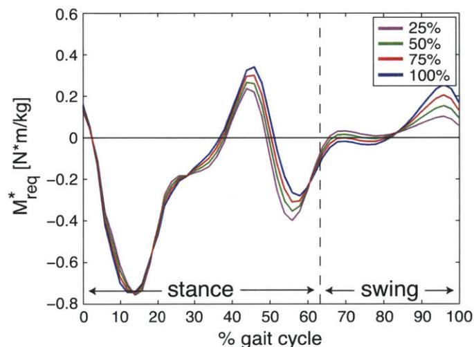
Figure 4-1: Gross effects of altering inertial properties on the knee moment required for a prosthetic leg to move with normative kinematics at a natural cadence.  $M_{req}^*$  is required knee moment normalized to body mass. The masses of all segments of the leg were scaled to the specified percentages of able-bodied values, and the moments of inertia (about the centers of mass of the segments) were scaled by the masses.
