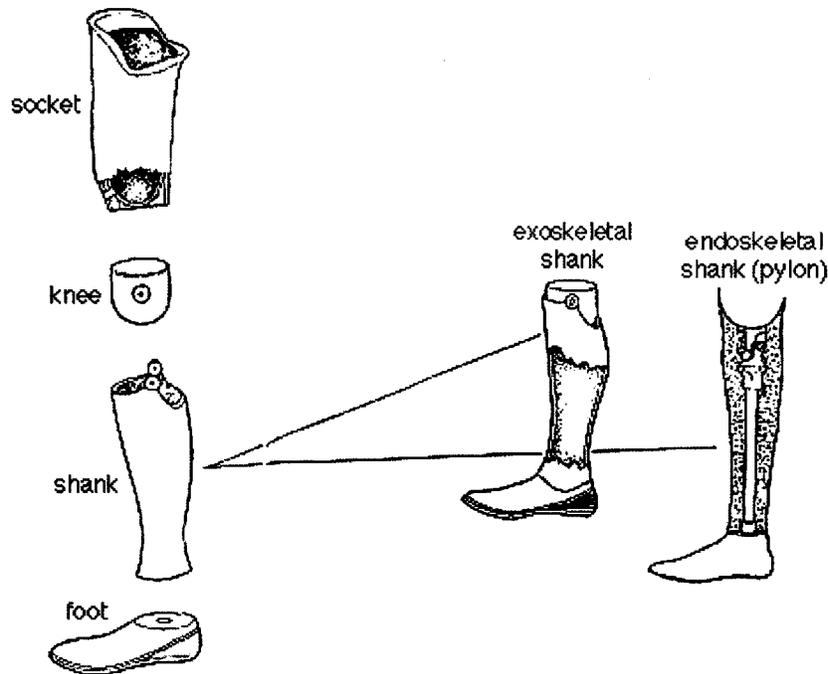
Figure 1-6: Drawing of a typical above-knee prosthesis. In an exoskeletal shank, load is borne upon a shell, whereas in an endoskeletal shank, load is borne primarily upon a pylon. As depicted, an endoskeletal shank may also have a cosmetic cover over the pylon. Adapted from [7].
