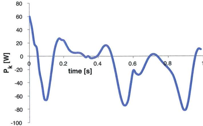
Figure 1-5: Knee joint power ( $P_k$ ) v. time over one gait cycle. Positive power is generated power, whereas negative power is dissipated power. Data adapted from Winter[5] for a 55.6 kg woman walking at a fast cadence.
