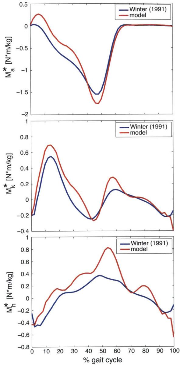
Figure 3-2: Comparison between moments calculated by model and moments reported by Winter (1991)[20] for walking at a natural cadence.  $M_a^*$  is ankle moment normalized to body mass,  $M_k^*$  is knee moment normalized to body mass, and  $M_h^*$  is hip moment normalized to body mass. From top to bottom,  $R^2 = 0.93$ ,  $0.91$ , and  $0.80$ .
