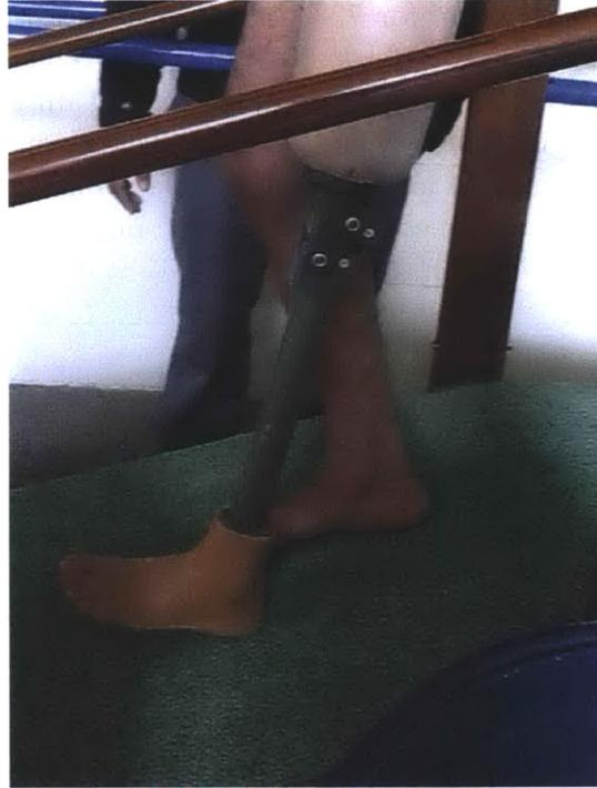
Figure 2-5: Photograph of the Stanford-Jaipur knee in a forcefully extended and lowered position. The subject walked down an incline and was initiating weight bearing on the prosthetic leg.
