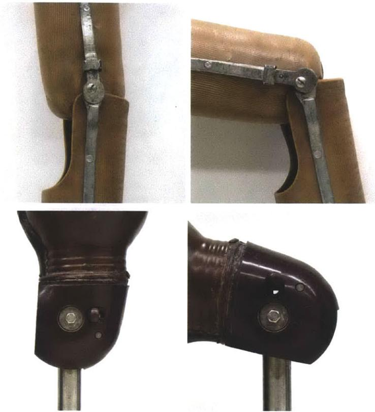
Figure 1-7: Two types of manual-locking knees. Top-left: BMVSS manual-locking knee, fully extended. Top-right: BMVSS manual-locking knee, flexed to nearly 90°. Bottom-left: ICRC manual-locking knee, fully extended. Bottom-right: ICRC manual-locking knee, flexed to nearly 90°.
