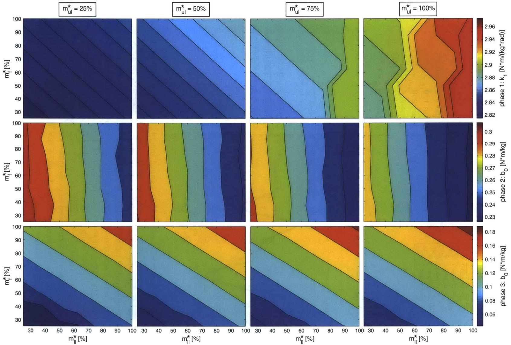
Figure 4-5: The effects of upper leg, lower leg, and foot mass on optimal MMC.  $m_{ul}^*$ ,  $m_{ll}^*$ , and  $m_f^*$  are upper leg mass, lower leg mass, and foot mass normalized to body mass.
