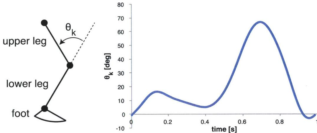
Figure 1-2: On left: convention used for knee joint angle ( $\theta_k$ ). Angular displacement in the positive direction is described as “flexion,” whereas angular displacement in the negative direction is described as “extension.” On right: knee joint angle v. time over one gait cycle. Peaks correspond to maximum flexion during loading response and maximum flexion during swing. Data adapted from Winter[5] for a 55.6 kg woman walking at a fast cadence.
