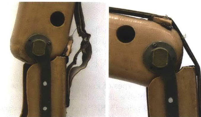
Figure 1-8: BMVSS single-axis free-swinging knee. On left: fully extended position. On right: flexed to nearly 90°. A band to resist excess flexion is visible at the front of the knee.
