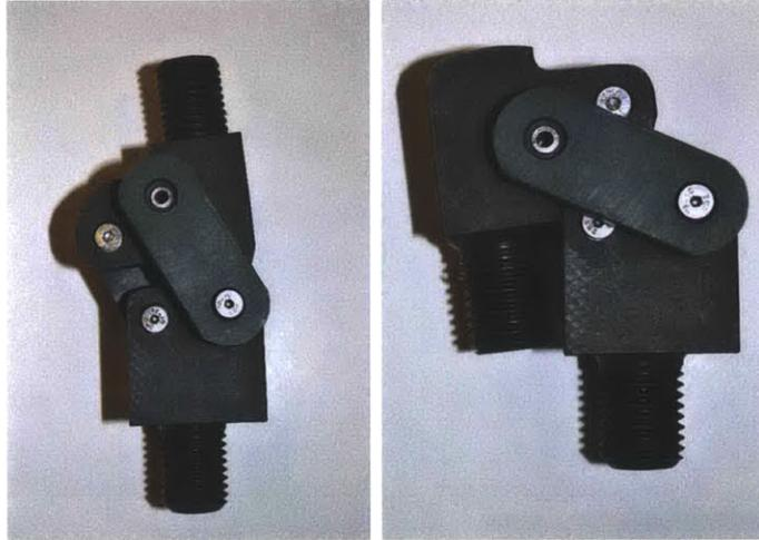
Figure 1-9: Stanford-Jaipur knee joint. On left: fully extended position. On right: fully flexed position.
