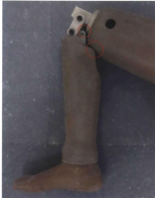
Figure 2-3: Illustration of squatting difficulties in a BMVSS above-knee prosthesis with the Stanford-Jaipur knee. Circled in red are collisions of 1) the socket with the shank and 2) the upper part of the knee with the lower part. Both collisions obstruct the deep flexion required for squatting.
