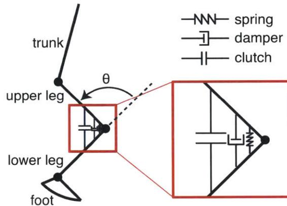
Figure 4-2: Schematic of general passive mechanical model used to model the knee.  $\theta$  is the knee angle.
