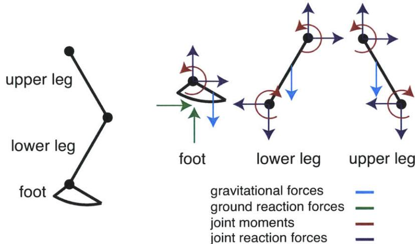
Figure 1-3: On left: sample 2-dimensional link-segment model for one leg. On right: free-body diagrams for all segments.
