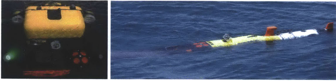
(a) HAUV - Ship hull inspection vehicle
