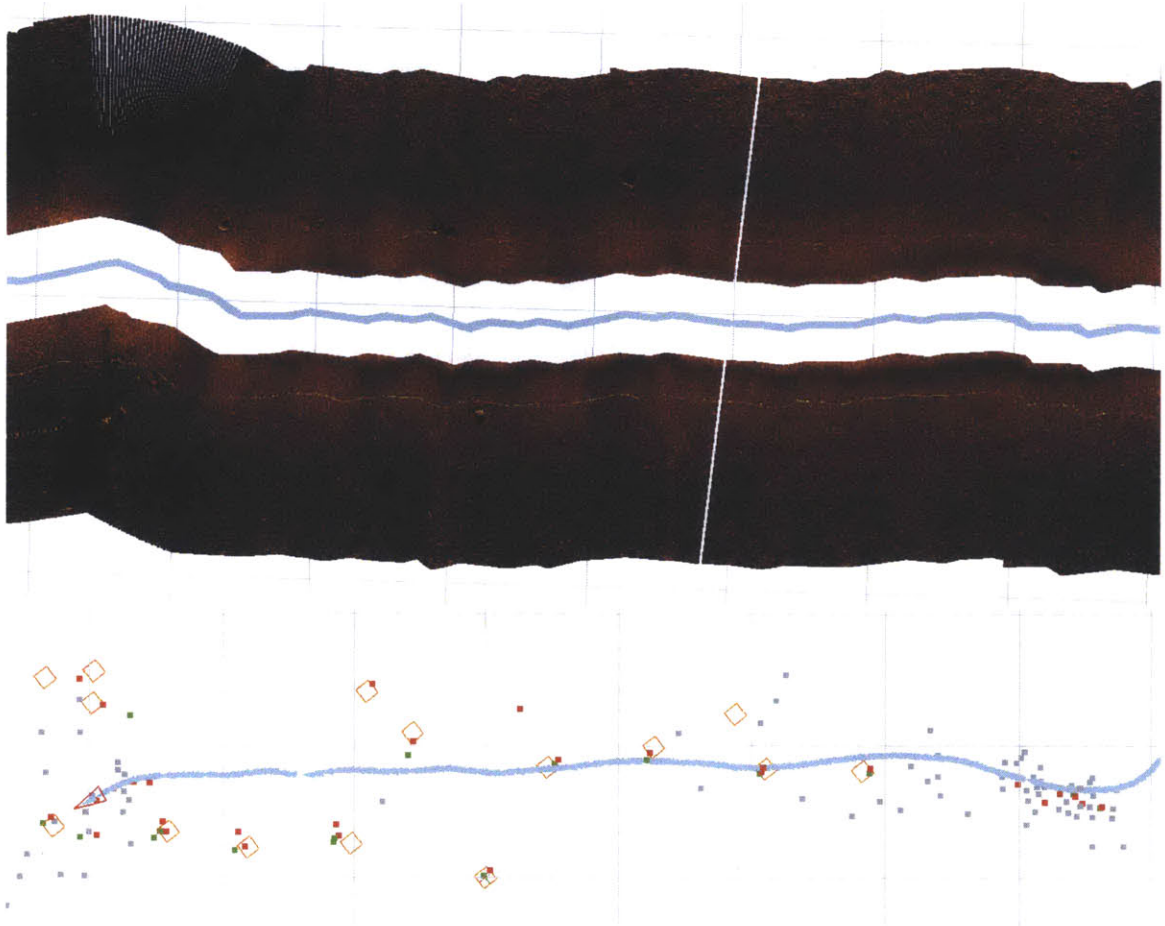
Figure 3-20: This figure shows the result of the estimated trajectory from the Panama City 2011 experiments. The boxes are objects identified from a previous mission. The green dots show the estimated position of features automatically detected in the forward looking sonar. The red points are features that did not get enough support.
