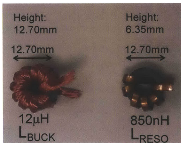
Figure 5-19: Customized L_{BUCK} and L_{RESO} inductors
