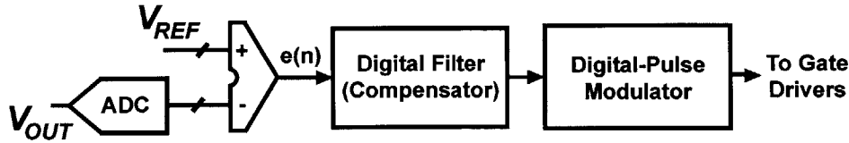
Figure 2-8: Block Diagram of a Digital Controller with ADC, Compensator and Digital Pulse Modulator [23]
