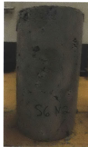
Figure 27: Concrete cylinder S6 No.2 post compression testing, still in one piece
