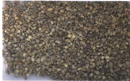
Figure 14: Coarse aggregate 0.371in group following separation
