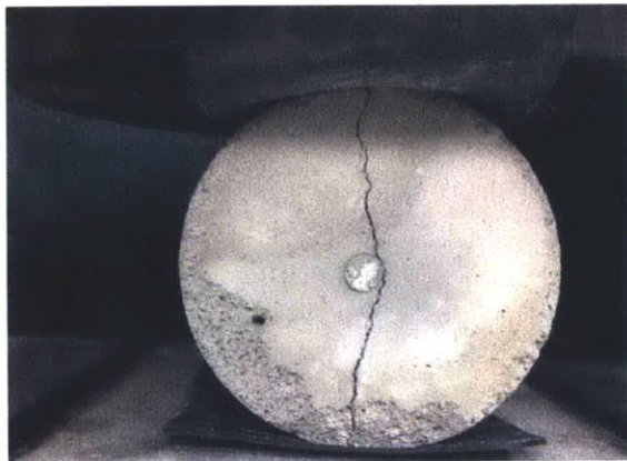
Figure 17: Concrete cylinder positioned with rubber supports during indirect tension test
