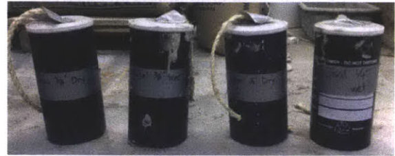
Figure 10: Fiber rope cylinder molds left to cure. Sisal 3/8" unsaturated, Sisal 3/8" saturated, Sisal 1/4" unsaturated, Sisal 1/4" saturated (left to right)
