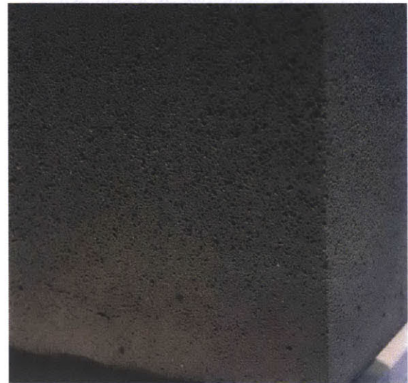
Figure 3: Varying density in a beam cast 5
