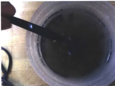
Figure 5: Hemp cut fibers with particulates floating to the top when stirred
