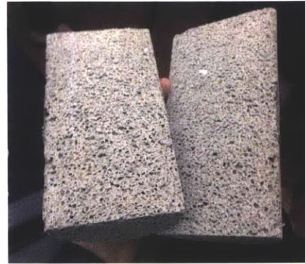
Figure 9: Sisal Mix 2 cylinder cut in half with the top closest to the camera lens
