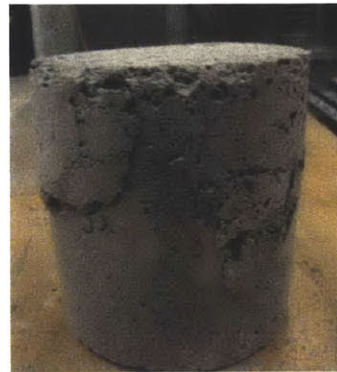
Figure 29: 0.25" aggregate concrete cylinder post compression testing
