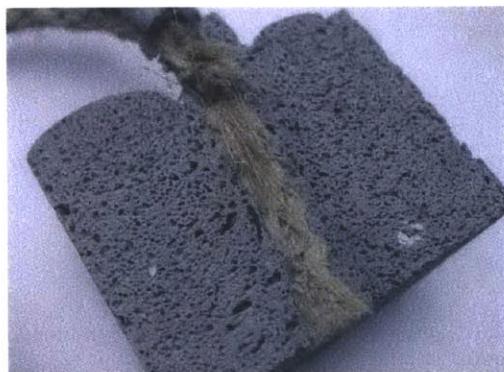
Figure 12: Saturated rope concrete cylinder sliced in half
