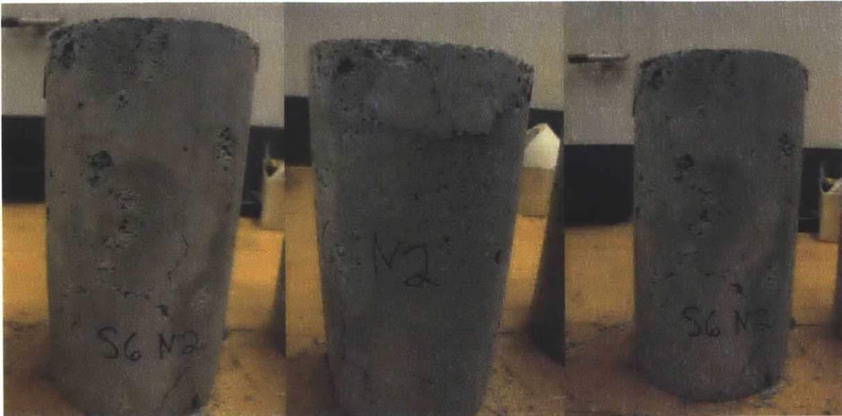
Figure 48: Cylinder S6N2 post compression testing
