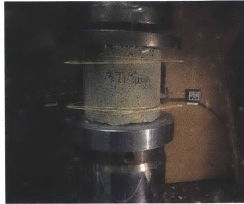
Figure 24: Concrete cylinder sample ready for compression loading
