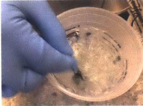
Figure 4: Stirring of cut sisal fibers in water
