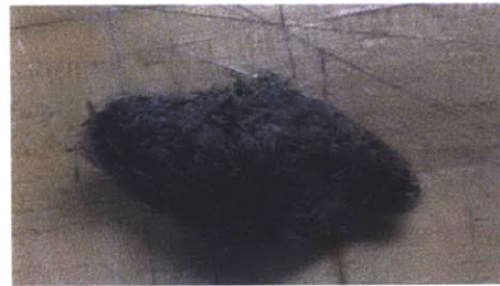
Figure 6: Compressed cut hemp fibers left to dry
