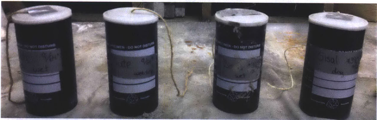
Figure 41: Fiber rope concrete cylinders left to cure (From left to right, Jute 9/64" saturated, Jute 9/64" unsaturated, Sisal #390 saturated, Sisal #390 unsaturated)
