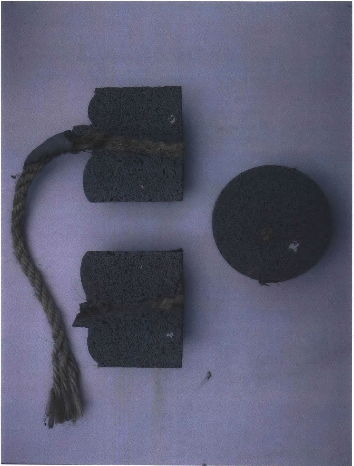
Figure 43: Saturated sisal fiber rope concrete cylinder
