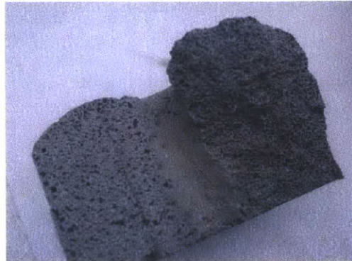
Figure 13: Unsaturated rope cylinder sliced in half after rope pulled from the cylinder
