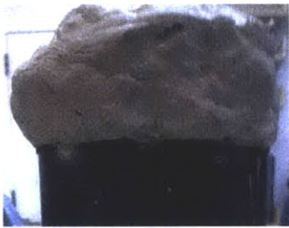
Figure 8: Early rising of graphite fiber test cylinder
