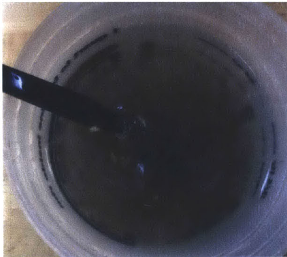
Figure 32: Jute No.1 mixing in water, noting particles floating to surface
