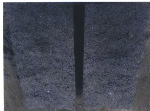
Figure 21: Cylinder S9 No.2 following the indirect tension test
