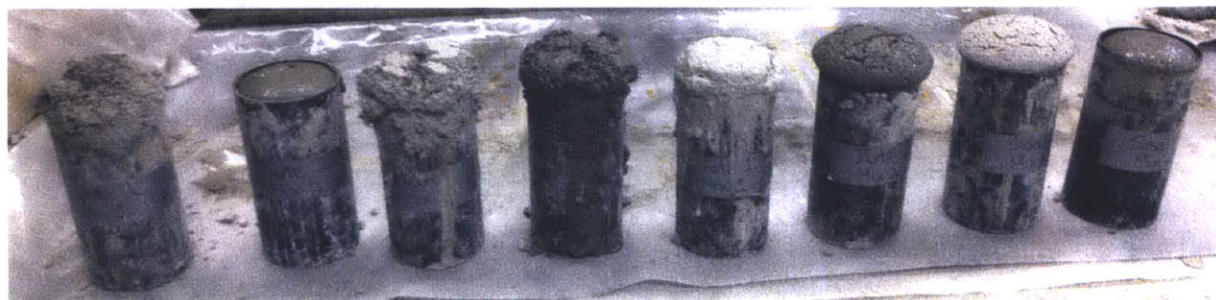
Figure 35: Natural cut fiber concrete mixes left to cure
