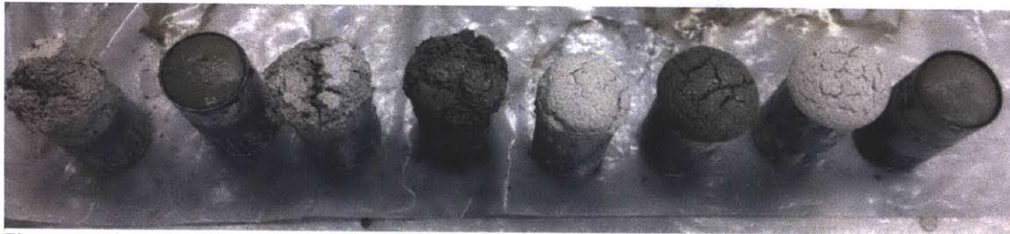
Figure 7: Fiber cut concrete cylinders left to cure. From left to right, Jute No. 2 Mix 1, Jute No. 2 Mix 2, Hemp Mix 1, Hemp Mix 2, Jute No. 1 Mix 1, Jute No. 1 Mix 2, Sisal Mix 1 and Sisal Mix 2.
