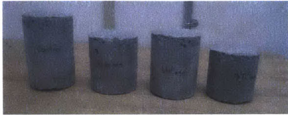
Figure 16: Fully cured and de-molded concrete cylinders (left to right, control, 0.187", 1/4" and 0.371")
