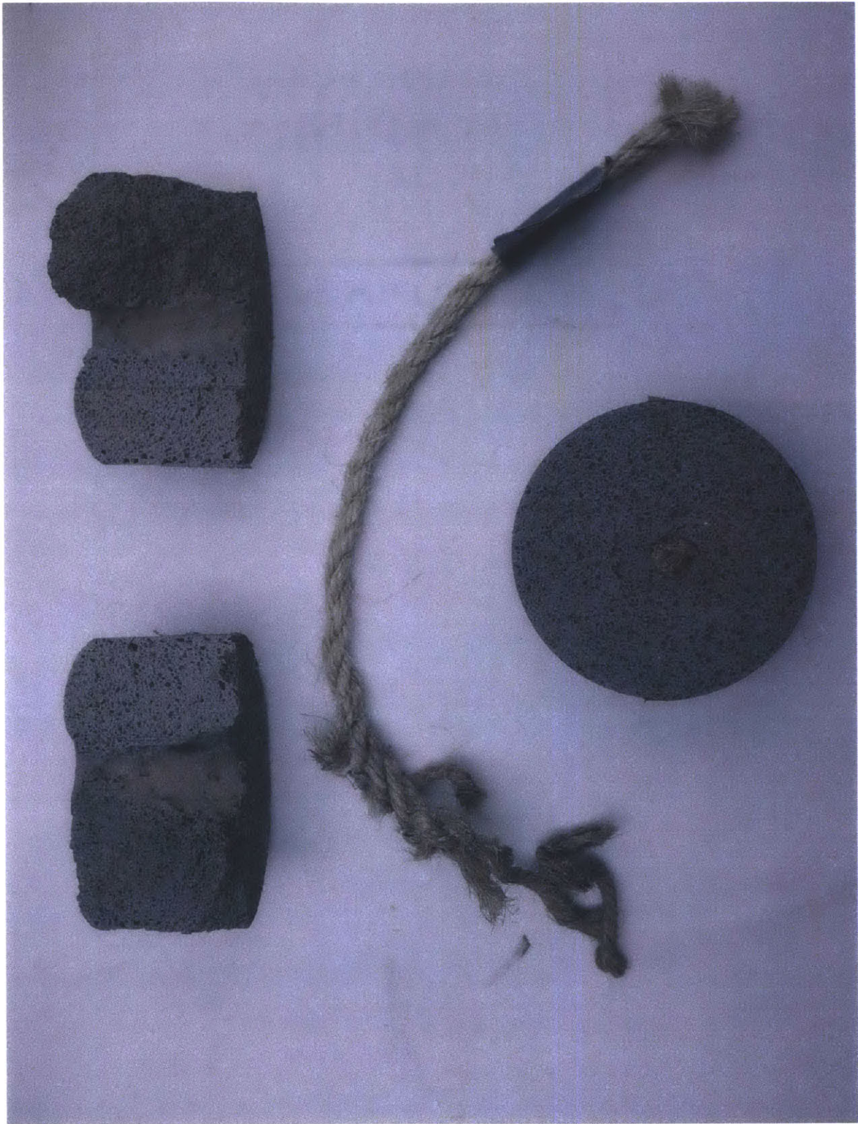
Figure 42: Unsaturated sisal fiber rope concrete cylinder
