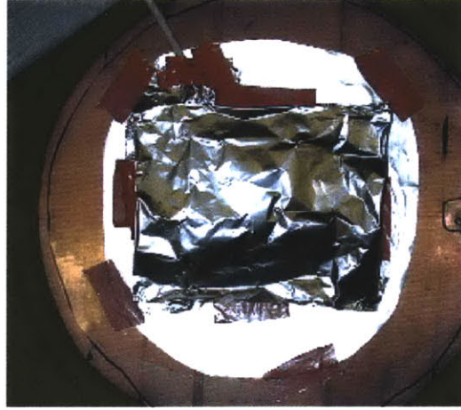
Figure 20: Foil Enclosure for EMI Shielding of PZT
