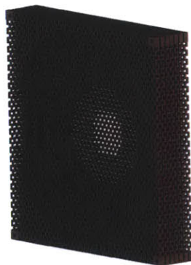
Figure 4-8: Solid model of the entire planoconcave lens made up of seven S-ring layers.
