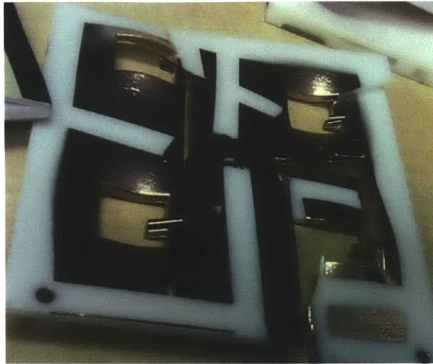
Figure 5-30: Conformal masks can be fragile, unable to withstand significant strains. In this image, a conformal mask broken while trying to remove it from the substrate. This mask included both a layer of Tango+ and a removable spray adhesive. The two together require a significant amount of force to separate the mask and substrate, resulting in mask damage.
