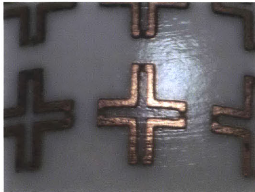
Figure 5-11: Close up of some copper cross unit cells deposited on the paraboloid dome. Note the deposition at the edge of the cross arms is noticeably light because of shadowing by the raised bridge on the conformal mask.
