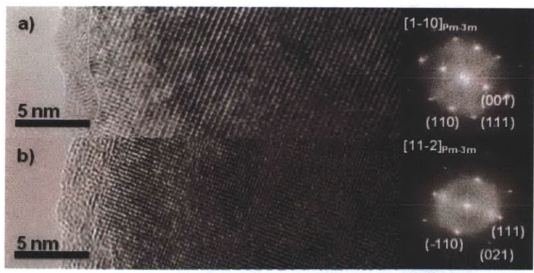
Figure 3.10: HRTEM and FFT of BSCF82 electrode that was cycled 5 times (a) with AB carbon and (b) without AB carbon. The amorphous layers are similar and show that AB carbon does not significantly contribute to the amorphization process. HRTEM performed by Christopher E. Carlton. Figure adapted from published work. 11
