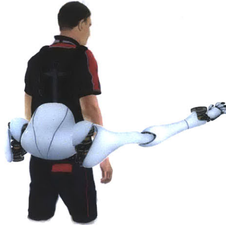
Figure 1-1: Concept drawing of the Supernumerary robotic limbs. Picture by F Parietti.
