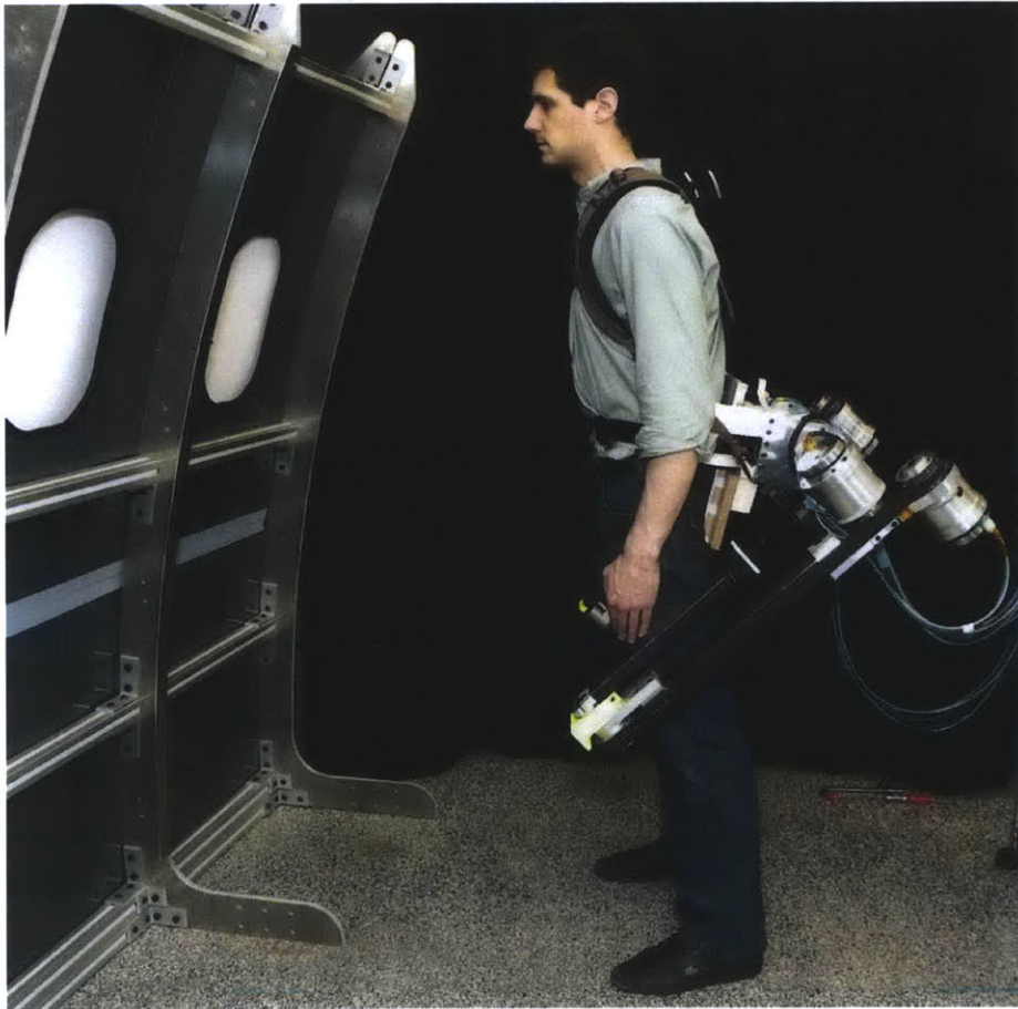
Figure 3-1: Supernumerary robotic limbs being worn by an operator. Picture by F Parietti and K Chan.
