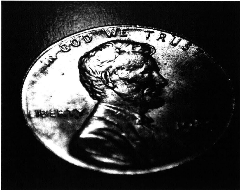
Figure 7-6: Example of Shortened X Resolution at Tilted Angle. This image was taken by our camera while tilted at a 45 degree angle with respect to the vertical axis. The naturally round penny now looks elliptical given the change in X resolution as the projection of the camera pixels onto the Cartesian coordinate frame is effected by the tilt angle.
