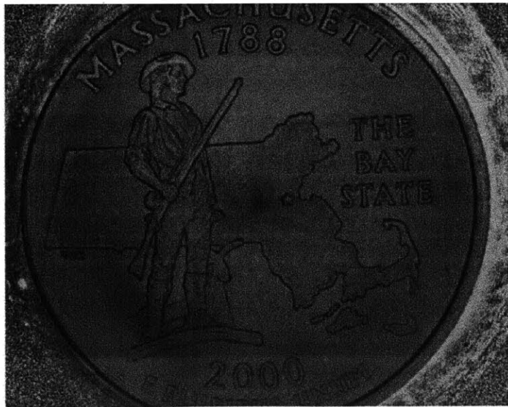
Figure 3-5: Improved Two Wavelength Imagery. This output shows the ratio of light between the two fluorescent liquids revealing a low noise image where intensity is proportional to thickness.
