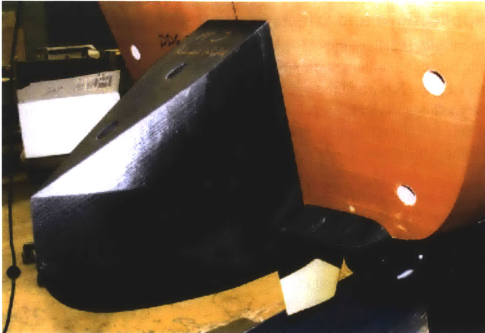
Figure 19: Example of a Stern End Bulb (Cusanelli and Karafiath 2012)
