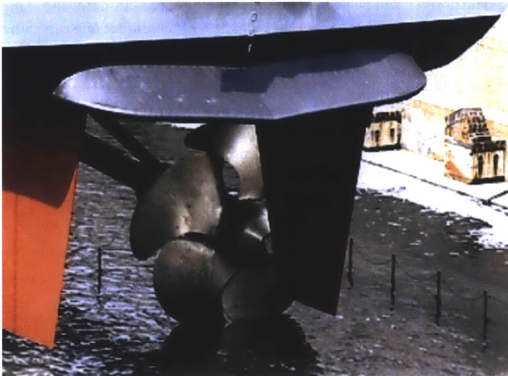
Figure 20: Example of a DDG 51 Stern Flap (Cusanelli and Karafiath 2012)
