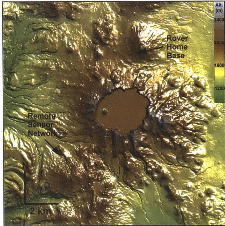
FIGURE 5-23. The Rover’s mission: deploy a distributed surface communications and sensing network between “Home Base” and the “Remote Site,” while maintaining at least periodic contact with the home base, and ensuring that each communications relay/sensor probe is network accessible. The rover must also plan its traverse so that it navigates around areas of steep terrain in order to stay on slopes less than 10 degrees.
