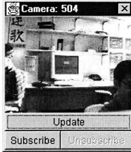
Figure 5-2: A screenshot from Camera . The display shows the latest image that has been received. Clicking the “Update” button will request the latest image from the camera, used in the request-response mode. The “Subscribe” and “Unsubscribe” buttons are for subscription-style interaction, where the camera sends an image using intentional multicast destined to all subscribers.
