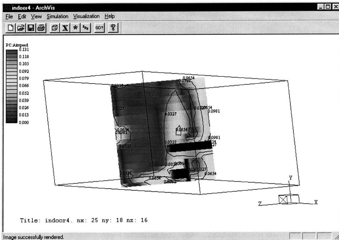
Figure 19: A contour plot of the airspeed of an indoor airflow model. The airspeed is also pseudocolored. Notice that the contour lines trace lines of similar color.
