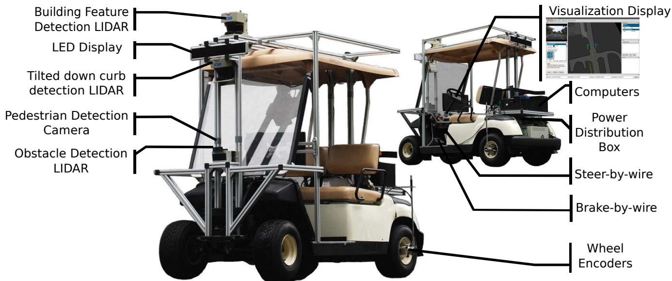
Fig. 1. Our vehicle testbed is built upon an electric golf car, augmented with a drive-by-wire system, and a small amount of sensors and computers.
