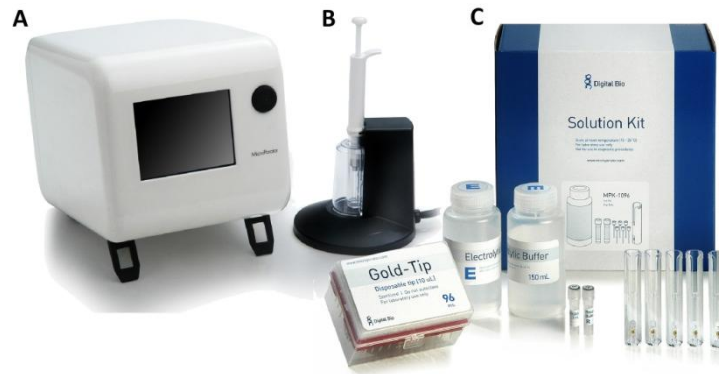
Figure 2.5: The Microporation System. (A) The Microporation unit that generates the electrical parameters necessary for electroporation which is transmitted to (B) the Microporation pipette dock consisting of a microporation tube containing electroporation buffer and the microporation pipette used to deliver electroporation to the cells through a gold plated pipette tip. (C) Microporation kit with all the necessary solutions, ( http://www.invitrogen.com/ ).
