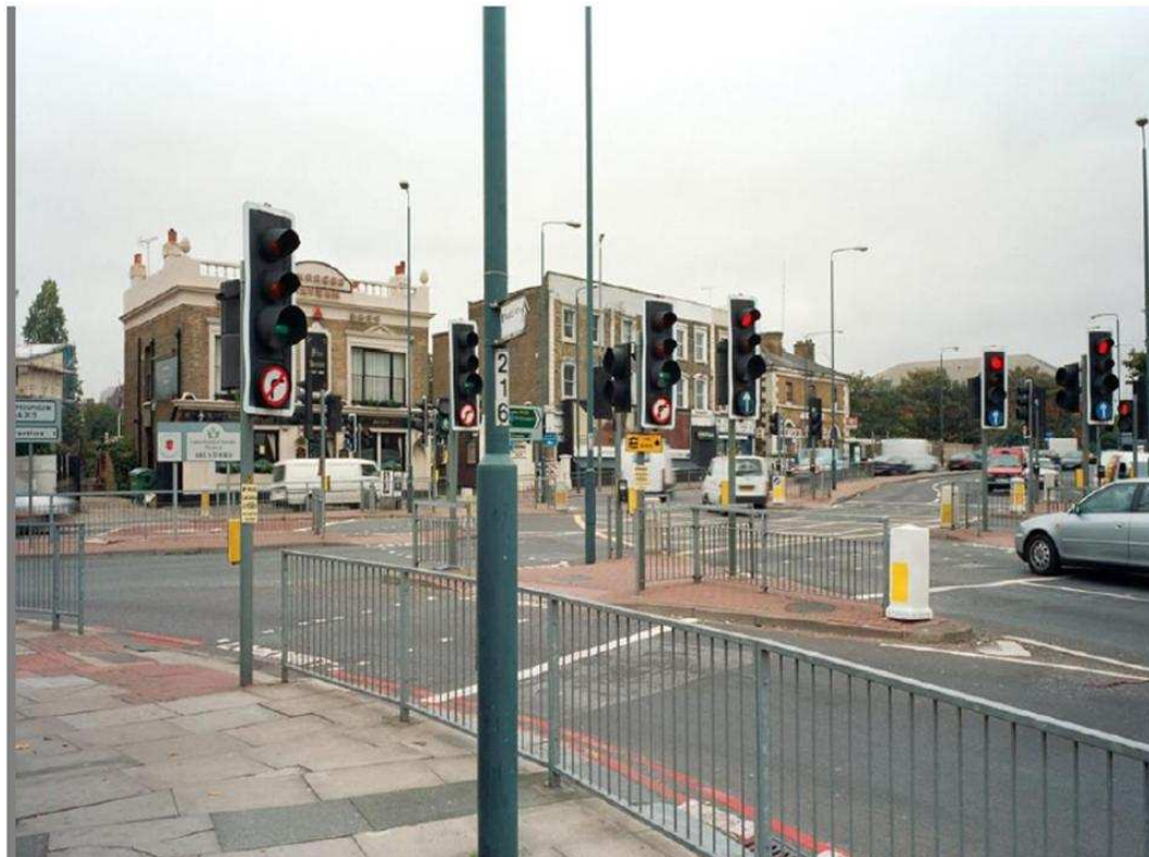
Figure 2-10: Cluttered Street with emphasis on features to segregate traffic from pedestrians (Source: Hamilliton-Ballie 2009)
