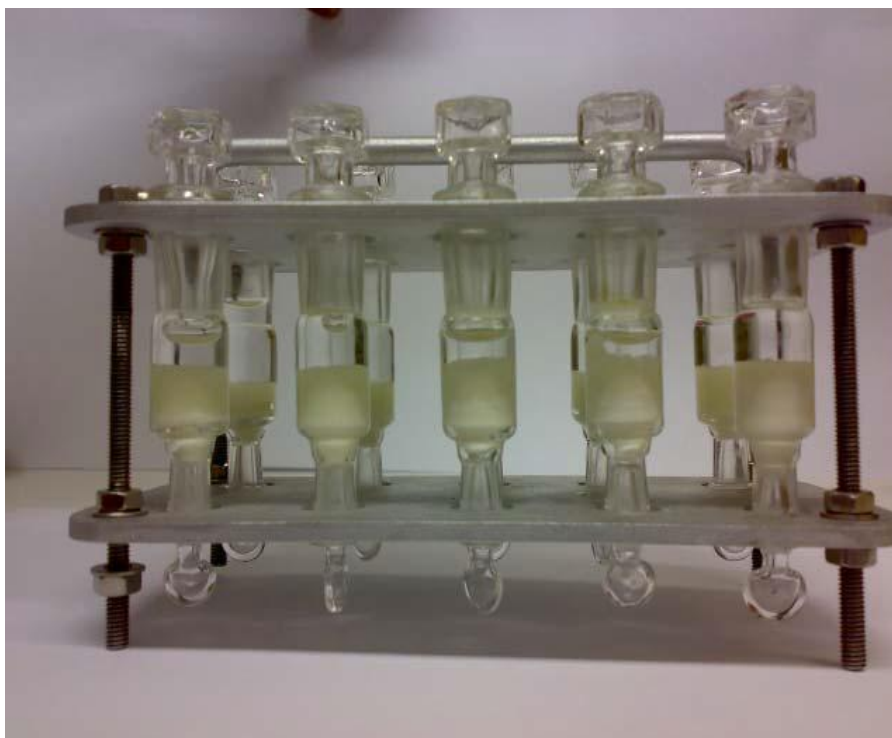
Figure 1.36: Glass discs 20 x 10 mm i.d. used as housings for monoliths prepared by ROMP and subsequent loading with PdNPs [53].
