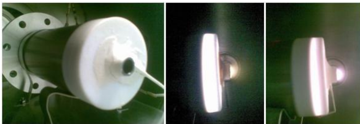
Figure 1: A view of a Constricted plasma source - A small hollow anode is mounted on the a hollow cathode aperture; (b) a hazy anode double glow (high anode voltage drop), (c) fully developed anode glow (minimum anode voltage drop)
