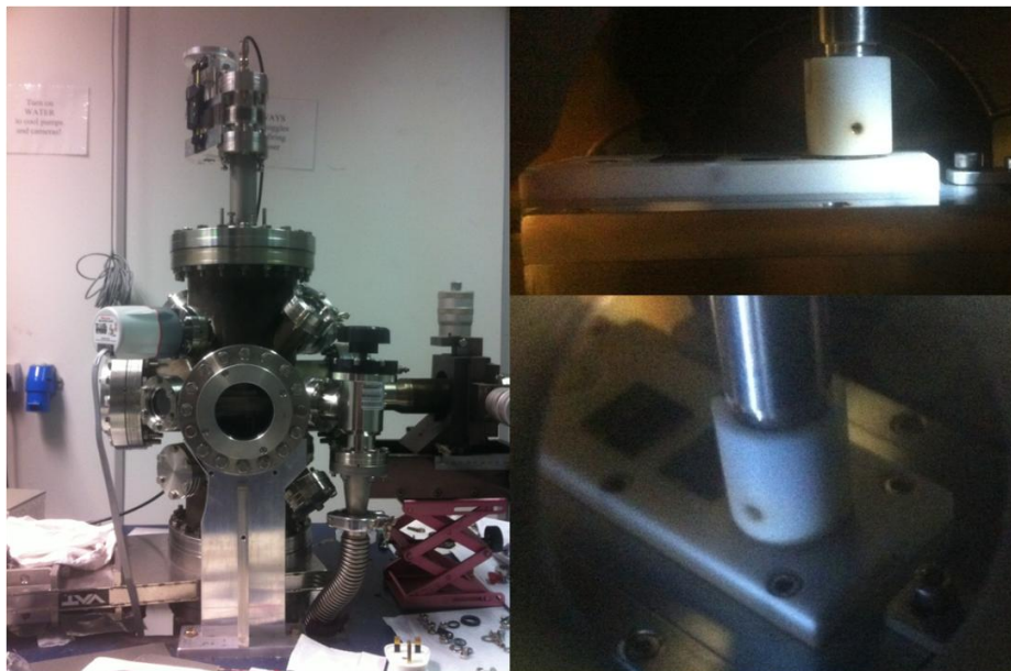
Figure 2.14: Photographs of FE chamber (left) and of the sample holder and movable electrode (right).
