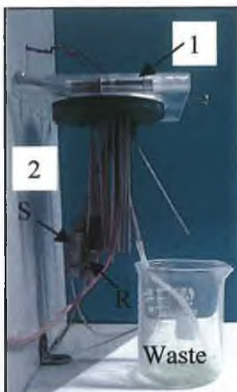
Figure 3-3 Side profile of the microfluidic chip holder including interconnects and optical detection
