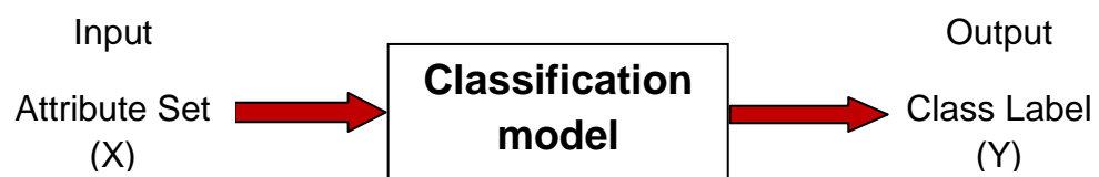
Figure 5-1 Classification as the task of mapping an input attribute set X into its class label Y.
