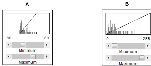
Figure 5-4: (A) illustrates the selection of minima and maxima in the intensity histogram of a positive nuclei object. (B) illustrates the equalised histogram after the remapping function.
