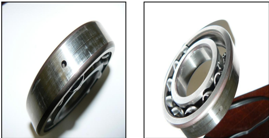
Figure 6.10 Faulted Bearing Before and After Test
