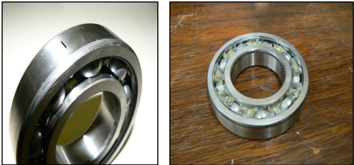
Figure 6.11 Re-greased Faulted Bearing
