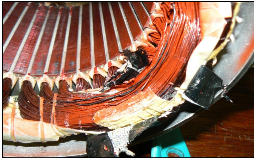
Figure 6.16 Stator Damage Due to Rubbing and Burnout
