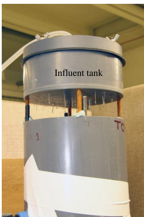
Unsaturated soil column influent application arrangement
