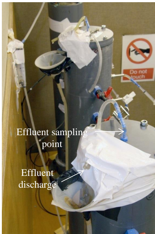
1 m saturated soil column effluent sampling and discharge arrangement
