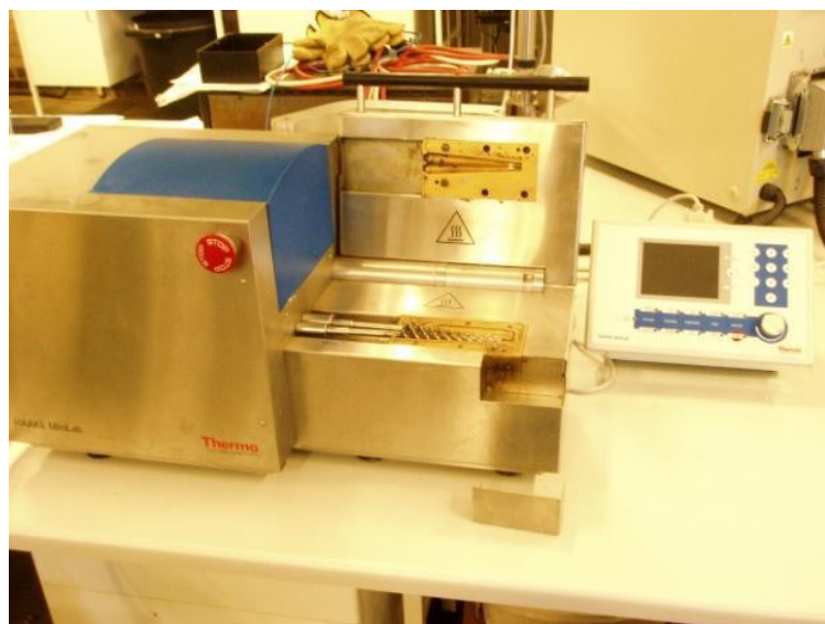
Figure 1.4: The Haake Minilab II Micro Compounder
