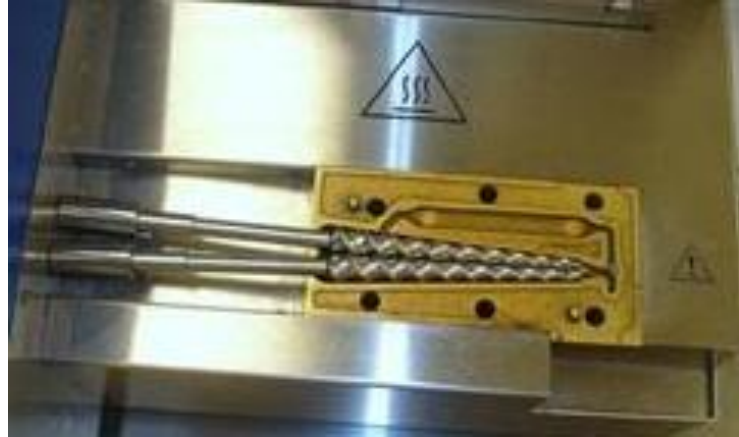
Figure 3.2: The limitation of commercial minimixer (unequal mixing history in recirculation channel).
