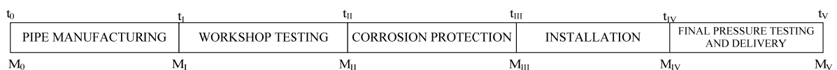
Figure 2 Milestones in a newbuilding ship pipeline manufacturing process Slika 2 Miljokazi u procesu izrade brodskih cjevovoda u projektu novogradnja
