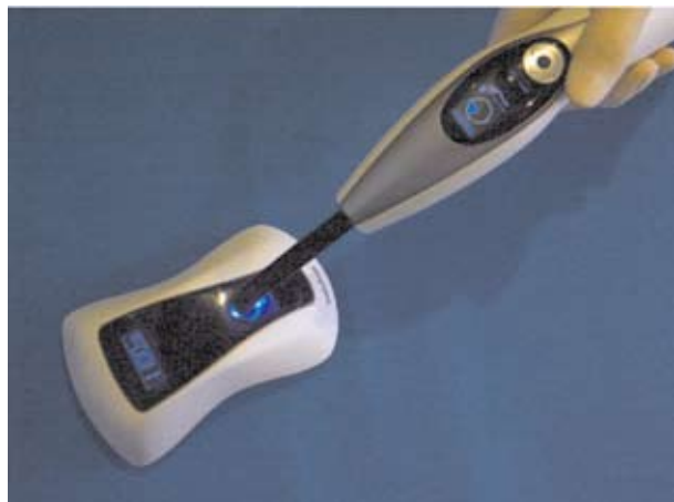
Fig. 1. Reading of light intensity by Bluephase meter.
