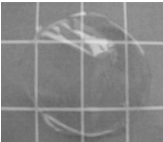
Fig. 1. A film obtained from crude exopolysaccharides of A. pullulans (the white lines at the background help seeing the transparency)
