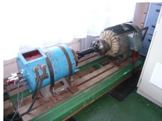
Fig. 3. Schematic diagram of the laboratory test bench and the photo of the traction drive system.
