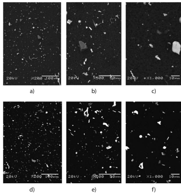
Figure 1 BEI micrographs of particles with: average contrast and brightness (a-c) and high contrast and maximum brightness (d-f)
