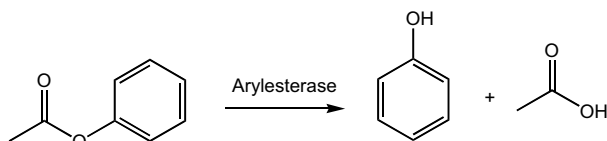
Scheme 1. Scheme of phenylacetate hydrolysis by arylesterase. Phenol, which absorbs at 270 nm, and acetic acid are obtained
