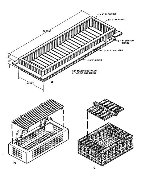
Figure 3. a) shedding box or float, Chesapeake Bay (illustration courtesy Steve Otwell) b) modern float constructed of fiberglass c) traditional southern crab float constructed of cypress
