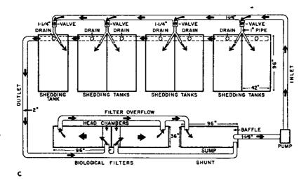
Figure 4. a) flow-through system or open system b) alternate placement of pump, open system c) closed system
