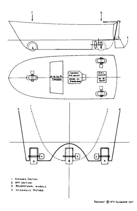
Figure 1. Lucander tunnel — hull design (upper figure: cross section; lower figure: plane view).
