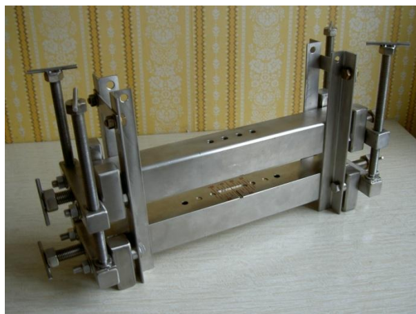
Fig. 1 Device for placing NdFeB magnets into two opposing assemblies
