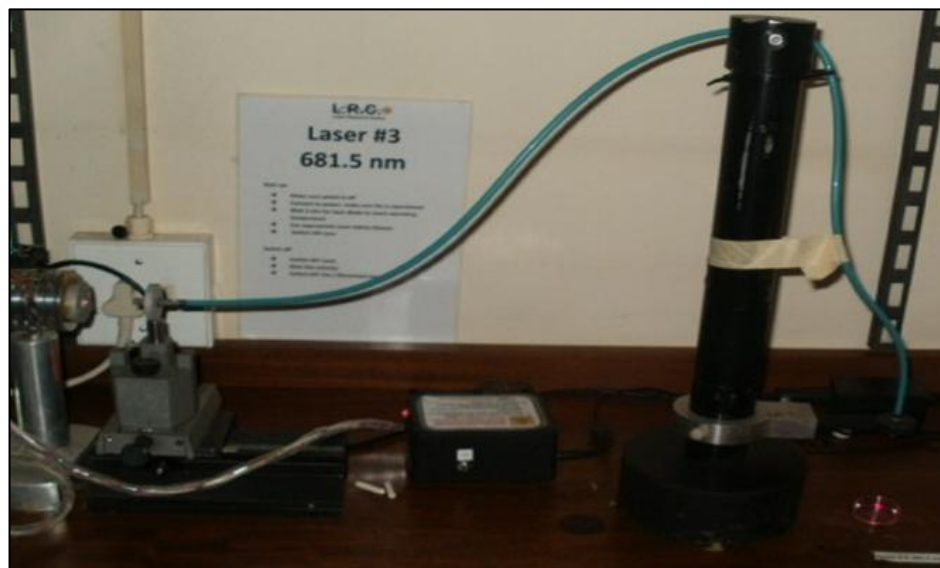
Figure 13 The 680 nm diode laser used to irradiate the human breast cancer cells.
