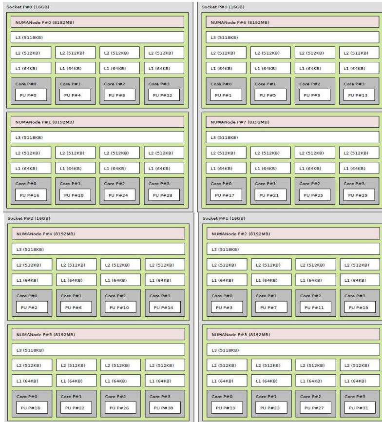
Fig. 7: Four sockets with two nodes. Each node has four cores.
