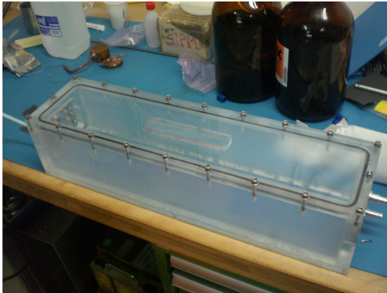
Figure 5.10 Plexiglass box realised for resolution measurements with a three-cell prototype.
