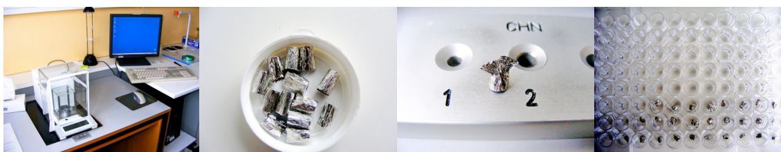
Figure 2 - From left to right: precision scale linked to PC, tin cups, firmly closed tin cups, final result (Pictures from Risø DTU Biosystems Department)
