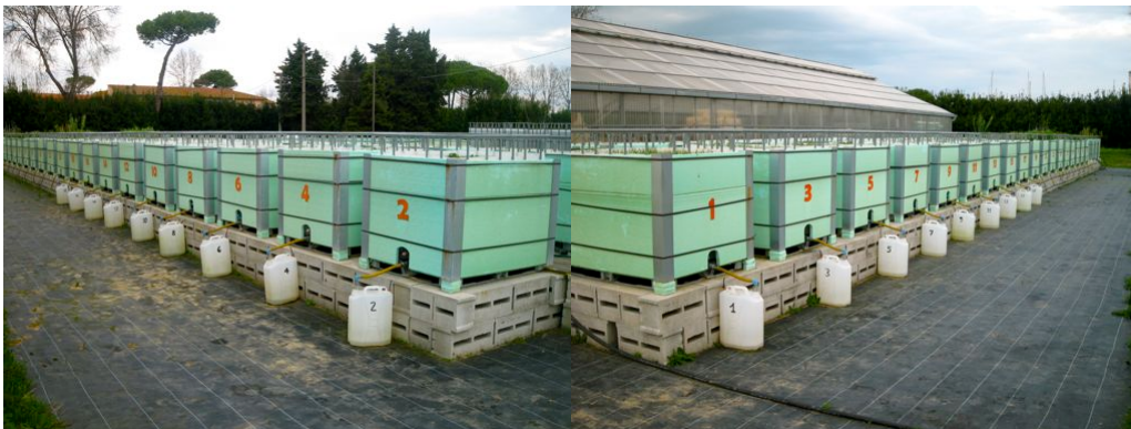
Figure 10 - Open-top lysimeters used for the experiment. Pictures taken at the Rottaia Experimental Station of the Dipartimento di Scienze Agrarie, Alimentari e Agro-ambientali of the University of Pisa (26/11/2009)
