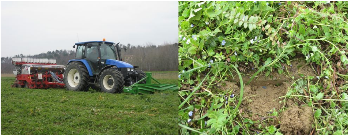
Figure 12 - Sod-seeding of sunflower ( Helianthus annuus L.) combined with a mechanical devitalization of a hairy vetch ( Vicia villosa Roth) cover crop (Pictures from an on-farm experiment in Lorenzana, Pisa)
